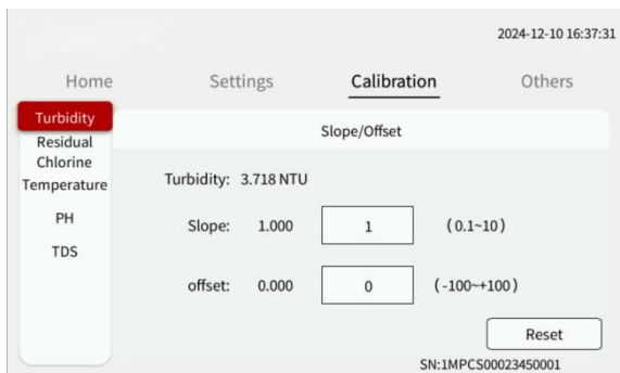
Fig.7 Calibration Diagram for Slope and offse
